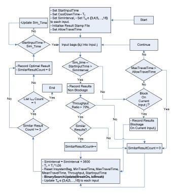
Figure 3: The embedded simulation optimisation algorithm.
