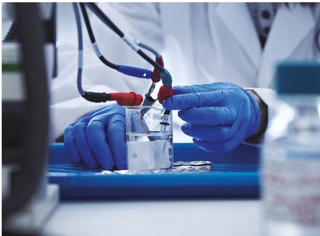
**Figure E3.** The author connects cables of a potentiostat to a three-electrode supercapacitor cell (the image is reproduced with permission from Deakin University).
