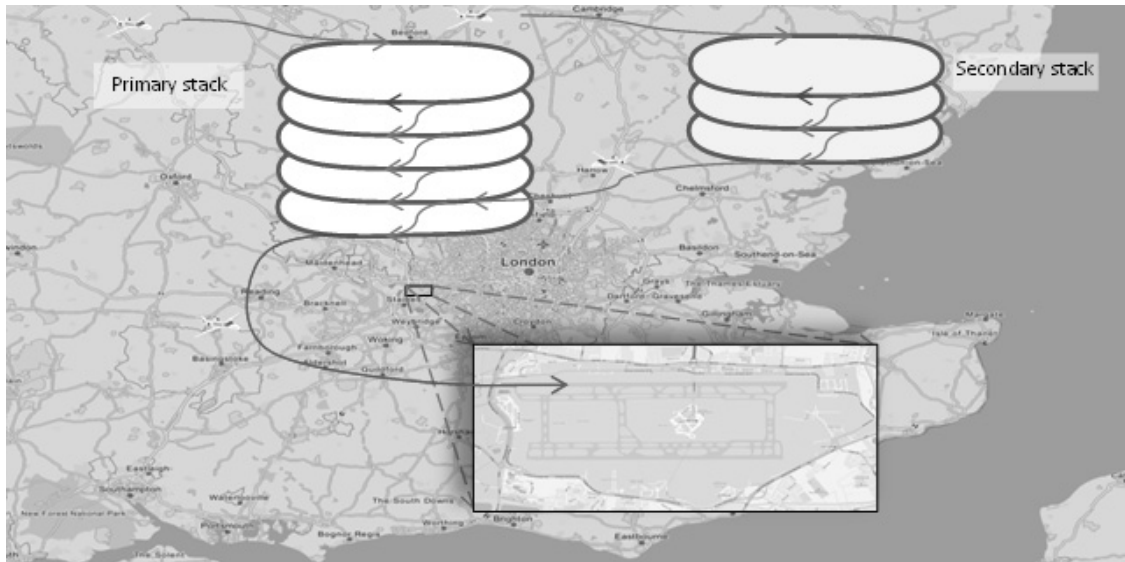
Figure 5.1: The solid lines describe how the aircraft act in non-emergency situations when they arrive to the airport while the runway is not yet available. When an aircraft arrives, it contacts the tower asking for landing permission. The tower evaluates the situation of all aircrafts then prioritises them, formerly it tells the aircraft to join a specific stack at a specified level until it receives the permission to land. In most of airports there exist 2 runways but only one is used for landing. The aircraft landing queue is represented in 2 stacks because of aerodynamics constraints.
